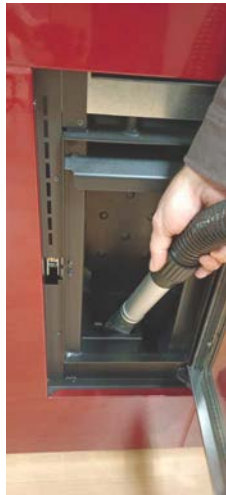
Fig. 36 - Burning pot box cleaning
